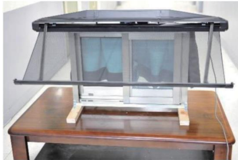
Fig. 7. (Color online) Electric sun shield.
