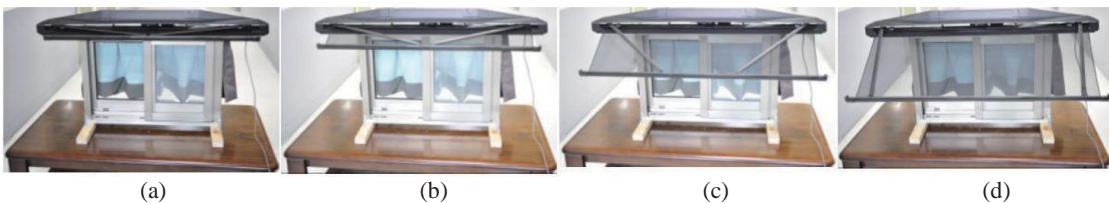
Fig. 11. (Color online) Electric sun shield in different states. (a) Disabled, (b) start to open, (c) open process, and (d) complete open.
